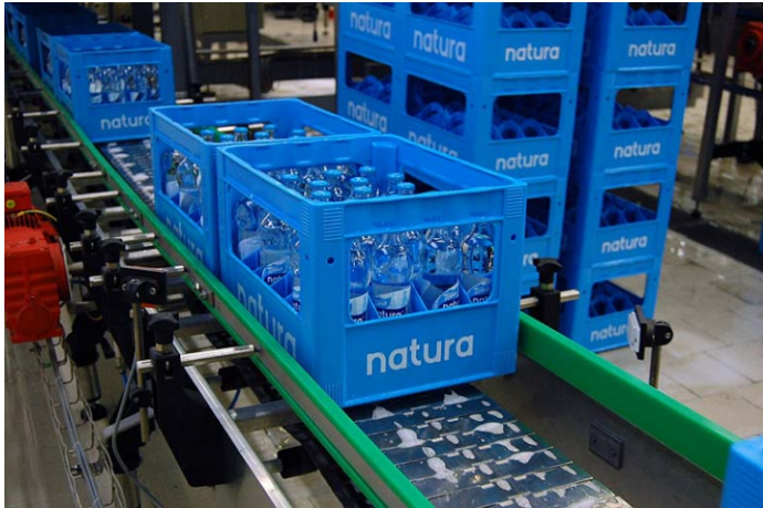
Case conveyors- PepsiCo, plant Toma Teplice nad Metují Czech Republic
